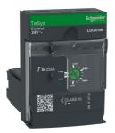
Standard control unit, TeSys Ultra, 4.5A to 18A, 3P motors, thermal magnetic protection, class 10, coil 24VAC
